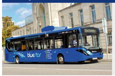
In 2018 we launched a trial in Southampton where we attached an air filter onto the top of a bus. When travelling through the city, this bus collected particulate matter in the air.
